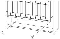
Figure 12 - Installing Bottom Mounting Screws
